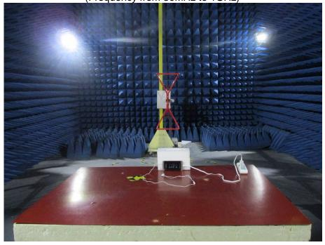
RADIATED EMISSION TEST (Frequency above 1GHz)
