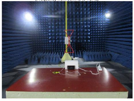
RADIATED EMISSION TEST (Frequency above 1GHz)
