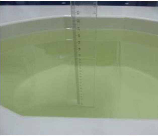
Photo 15: 1800~1900MHz Liquid Depth \geq 15.0cm
