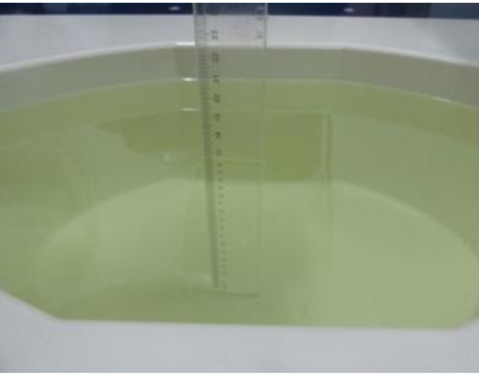
Photo 16: 2450MHz Liquid Depth \geq 15.0cm
