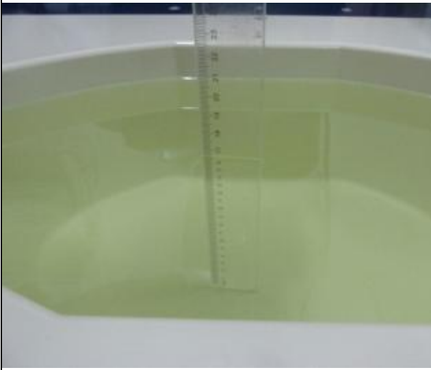
Photo 15: 1800~1900MHz Liquid Depth \geq 15.0\text{cm}
