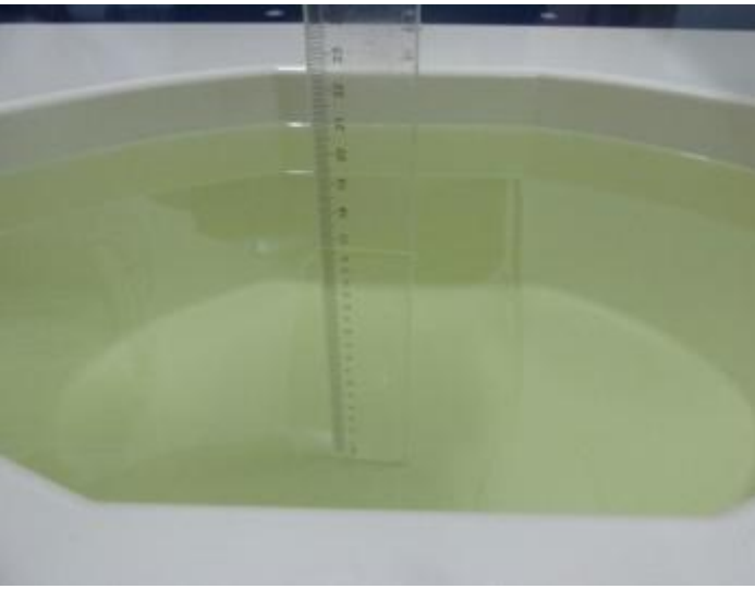
Photo 16: 2450MHz Liquid Depth \geq 15.0\text{cm}
