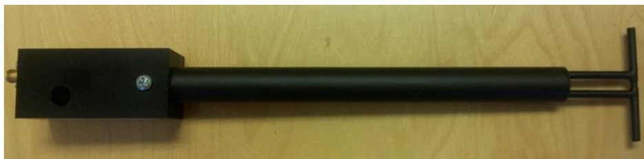
Figure 1 – MVG COMOSAR Validation Dipole
