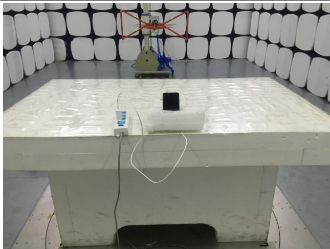
Conducted Emissions Test Setup Front View
