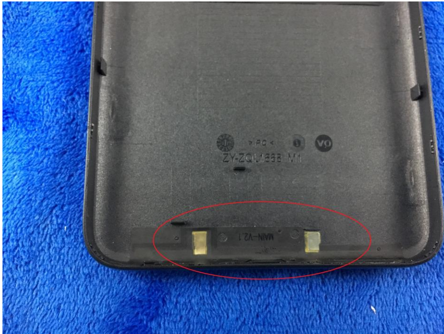
GSM/PCS/U MTS-FDD/LTE Antenna View
