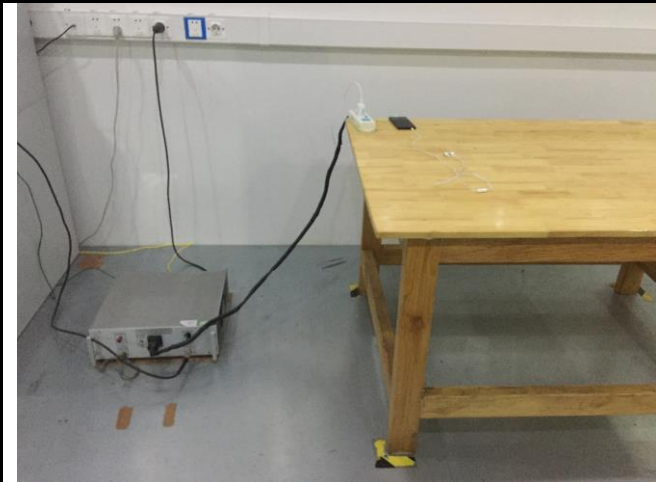
Conducted Emissions Test Setup Front View
