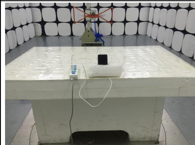
Conducted Emissions Test Setup Front View
