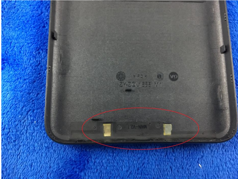
GSM/PCS/U MTS-FDD/LTE Antenna View
