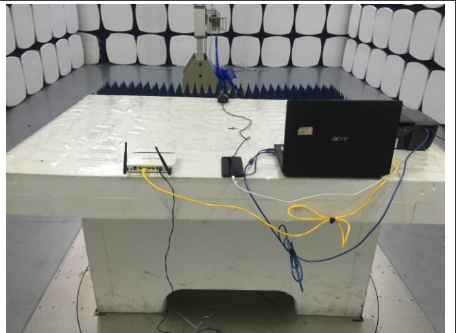
Radiated Emissions Test Setup Above 1GHz
