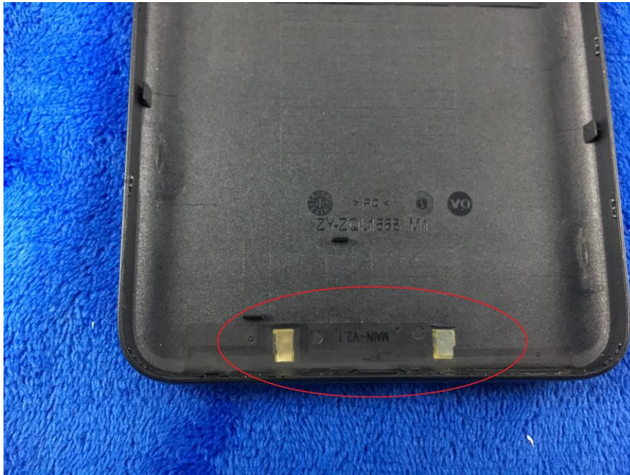
GSM/PCS/U MTS-FDD/LTE Antenna View
