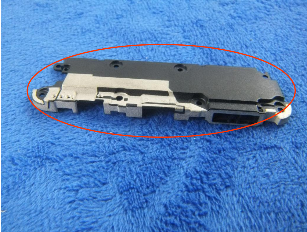
GSM/PCS/UMTS-FDD Antenna View
