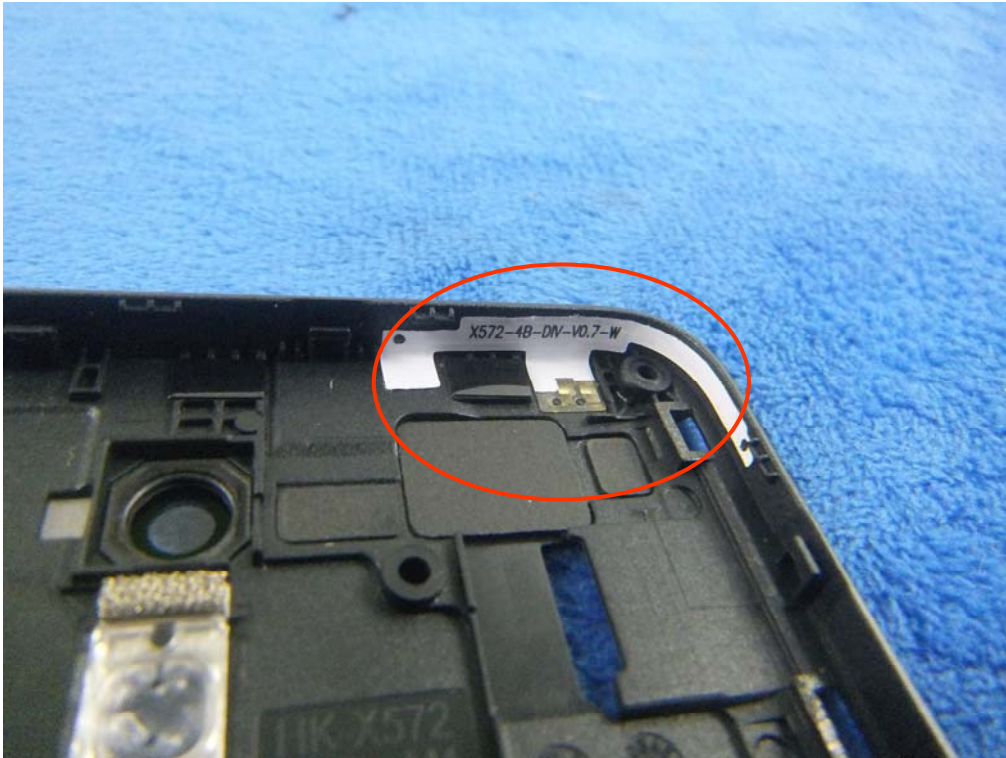
LTE - Antenna View
