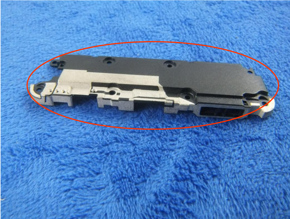
GSM/PCS/UMTS-FDD Antenna View
