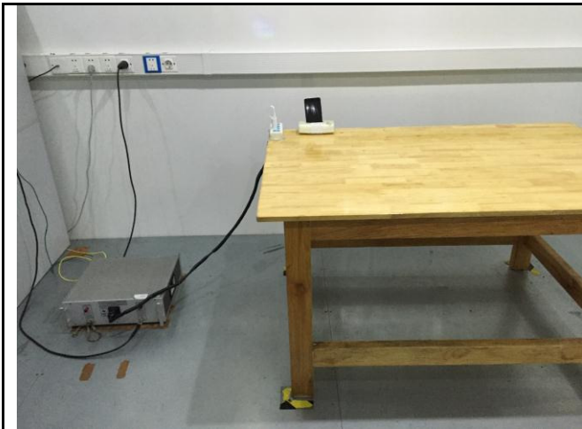
Conducted Emissions Test Setup Front View
