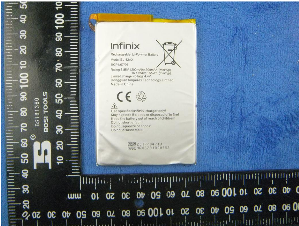
Battery - Rear View
