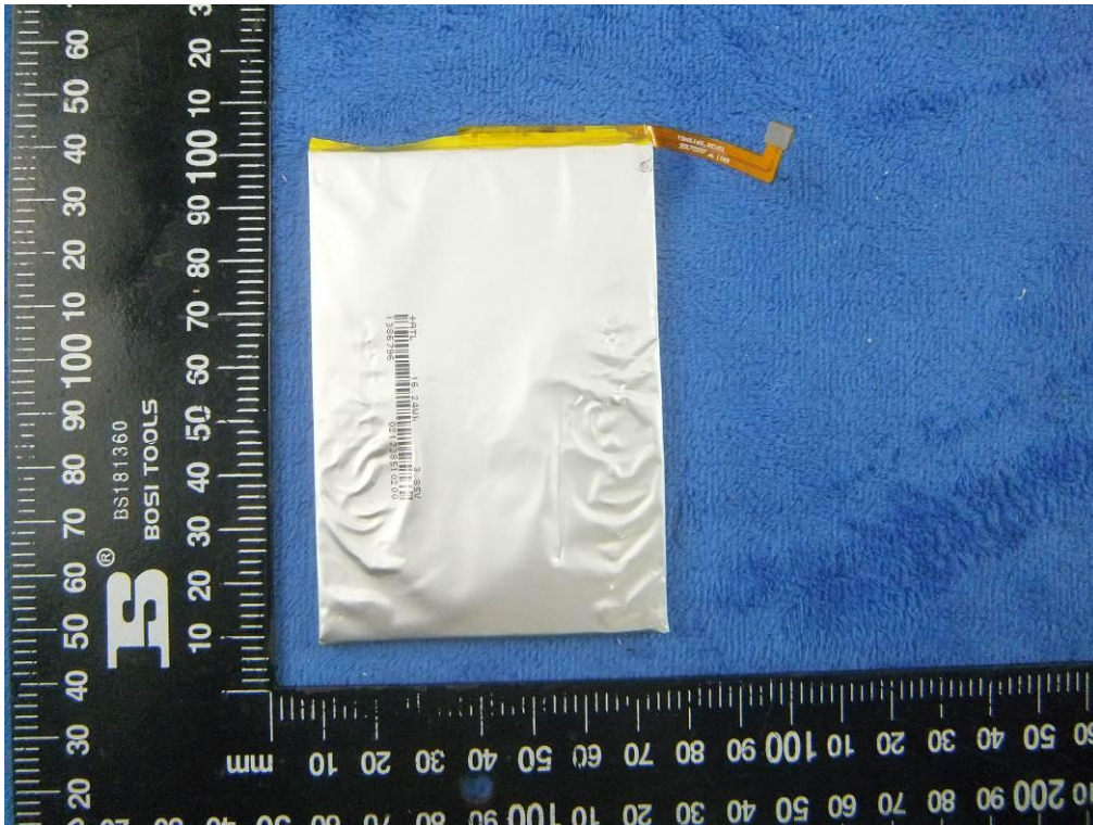
Battery - Front View
