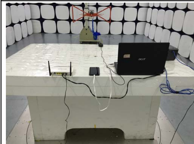
Conducted Emissions Test Setup – Front View
