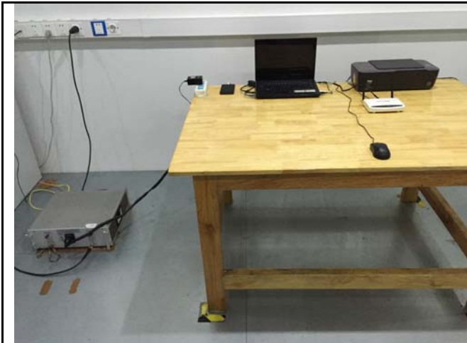
Conducted Emissions Test Setup – Front View
