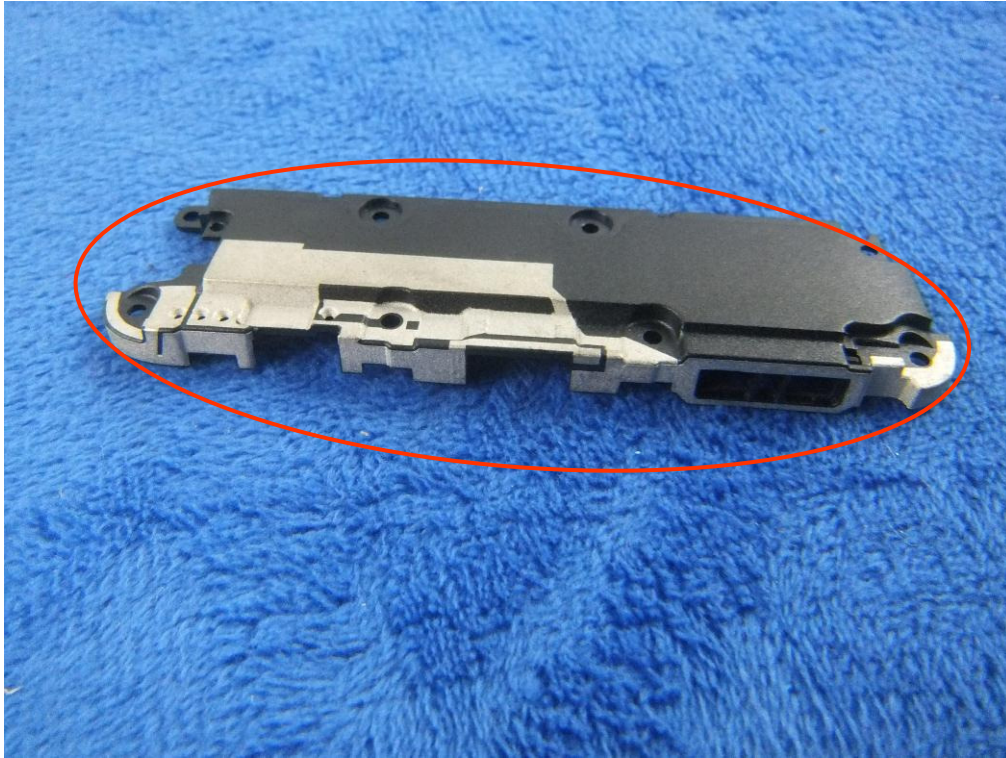
GSM/PCS/UMTS-FDD Antenna View
