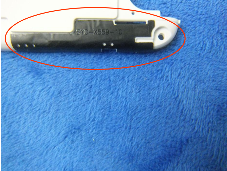
GSM/PCS/UMTS - Antenna View
