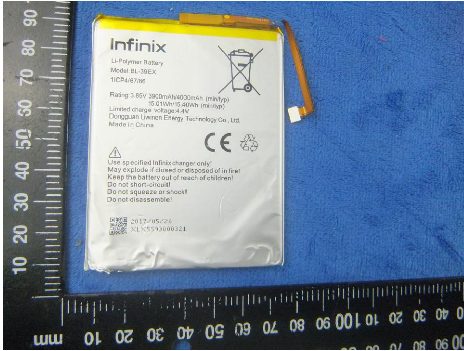
Battery - Front View
