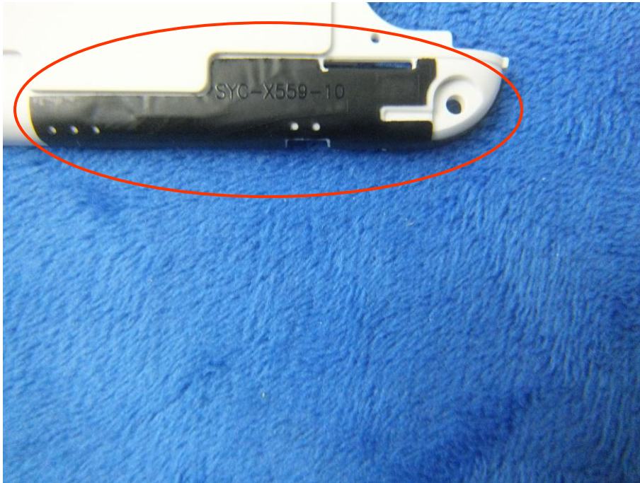
GSM/PCS/UMTS - Antenna View
