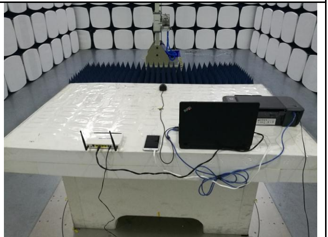
Radiated Emissions Test Setup Above 1GHz
