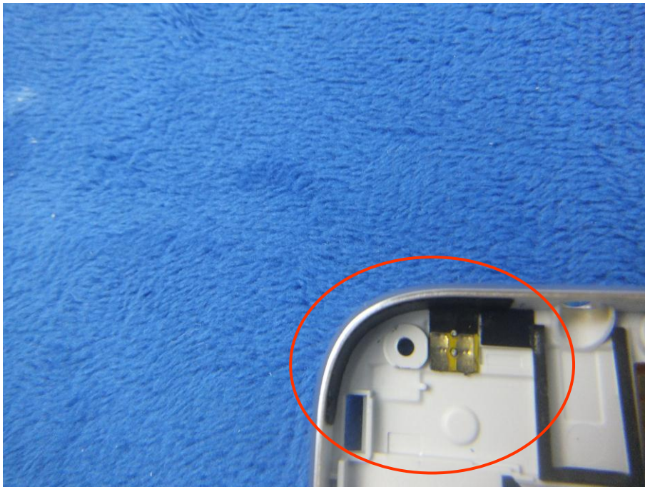
BT/WIFI - Antenna View
