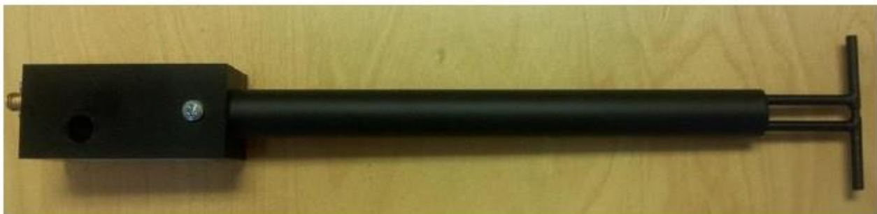
Figure 1 – MVG COMOSAR Validation Dipole
