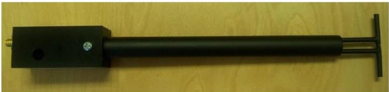
Figure 1 – MVG COMOSAR Validation Dipole
