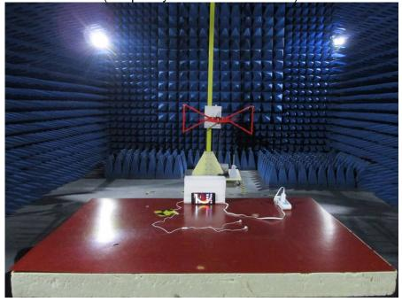
RADIATED EMISSION TEST (Frequency above 1GHz)
