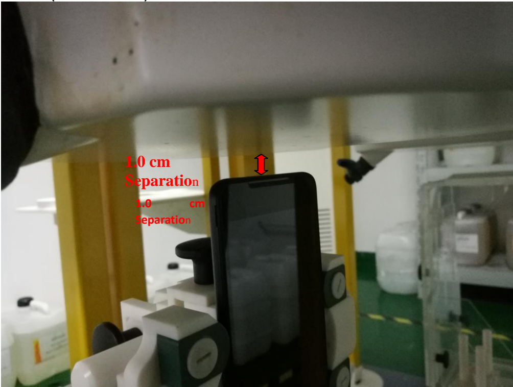
Body Setup Photo (LCD BOTTOM)
