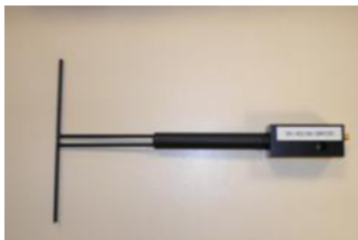
Figure 1 – Satimo COMOSAR Validation Dipole
