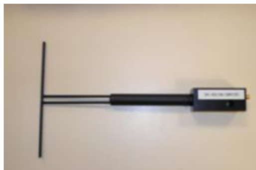
Figure 1 – Satimo COMOSAR Validation Dipole
