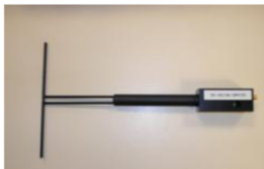
Figure 1 – Satimo COMOSAR Validation Dipole
