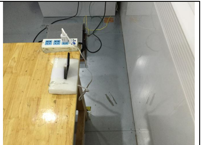
Conducted Emissions Test Setup Side View
