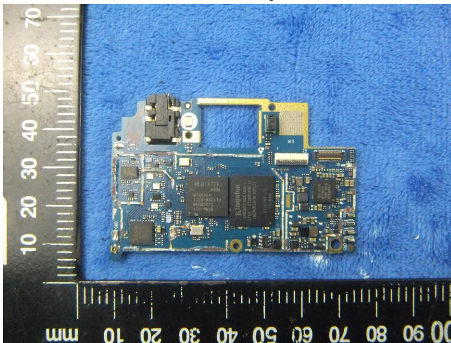
Mainboard without Shielding - Front View
