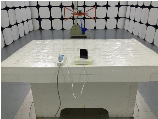
Conducted Emissions Test Setup Front View
