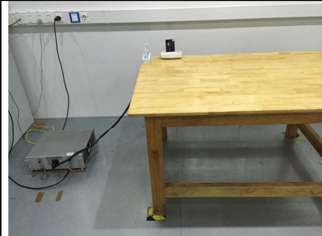
Conducted Emissions Test Setup Front View
