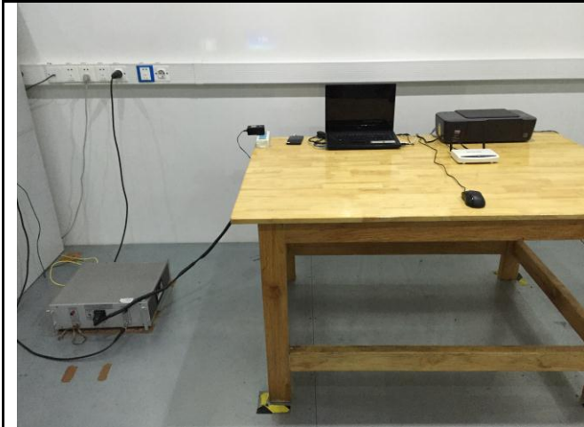
Conducted Emissions Test Setup – Front View
