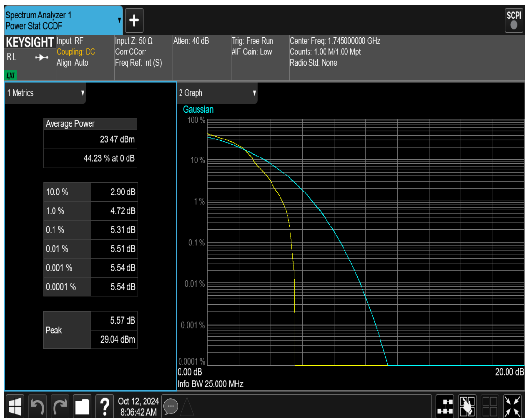
Band66 QAM16 BW=15MHz Channel=132322 RB Size=1 Position=#0
