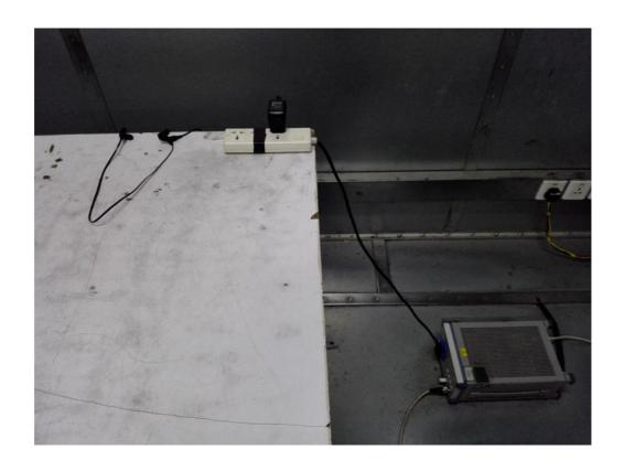
Radiated Emission Test
