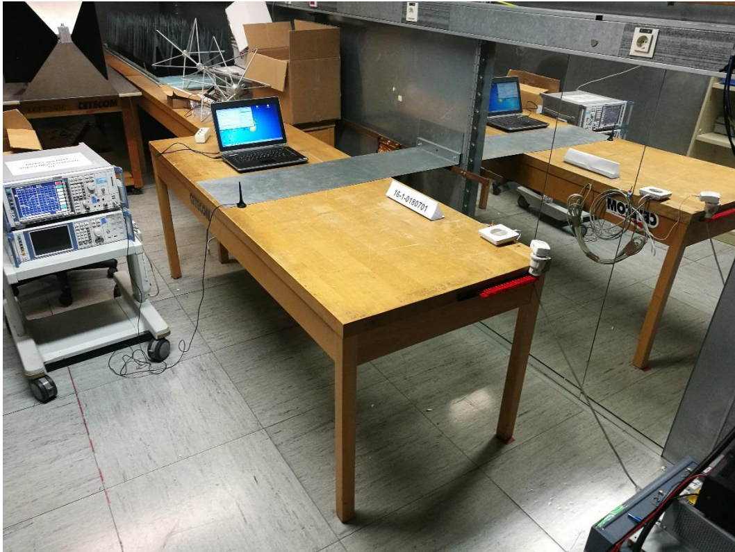
Photograph 19: Set Up 2-Overall View -WLAN 2.4 GHz Tests- AC-Power Lines Emissions
