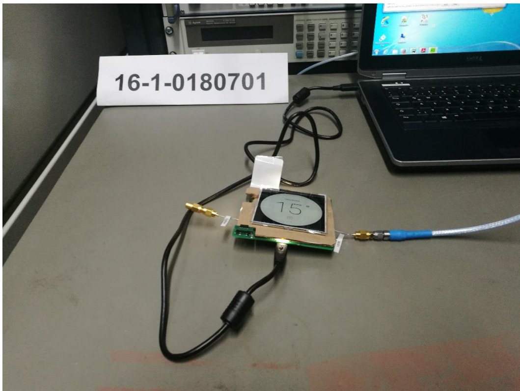
Photograph 4: Set Up 1-Close View -WLAN 2.4 GHz Tests- RF Power + Duty Cycle+ PSD + 6 dB BW
