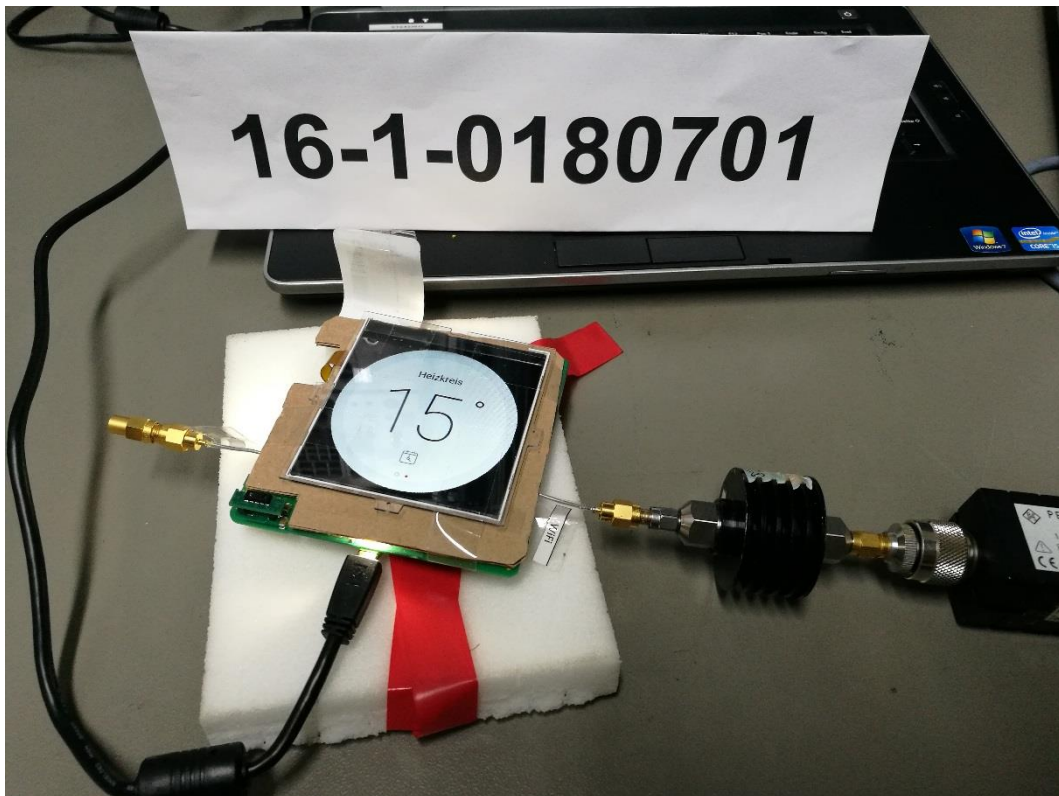
Photograph 2: Set Up 1-Close View -WLAN 2.4 GHz Tests- Power Verification
