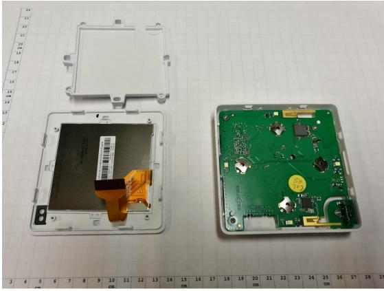
Photograph 3: ViCare Thermostat – Housing Top Side – Display Back
