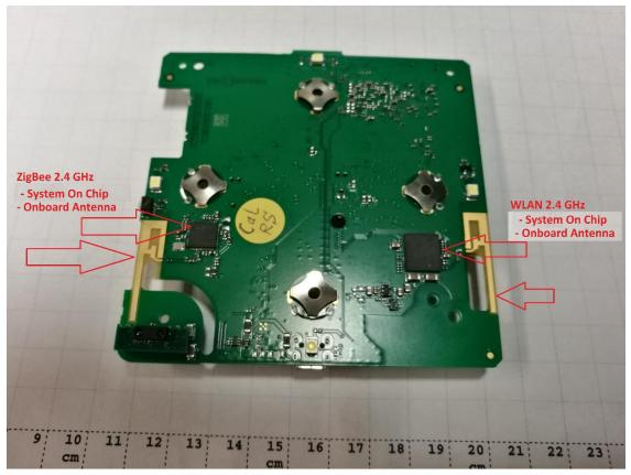
Photograph 8: ViCare Thermostat – Radio Modules + Onboard Antennas
