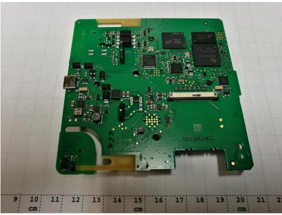
Photograph 6: ViCare Thermostat – Main PCB Bottom Side
