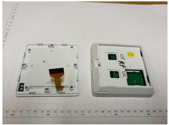
Photograph 2: ViCare Thermostat – Housing Bottom Side
