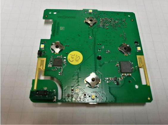
Photograph 5: ViCare Thermostat – Main PCB Top Side
