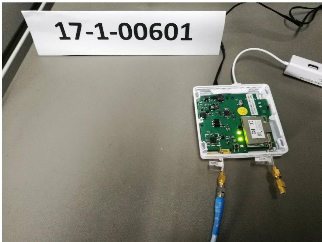
Photograph 2: Set Up 1-Close View - ZigBee 2.4 GHz Tests- RF Power + Duty Cycle + PSD +6 dB B.W.
