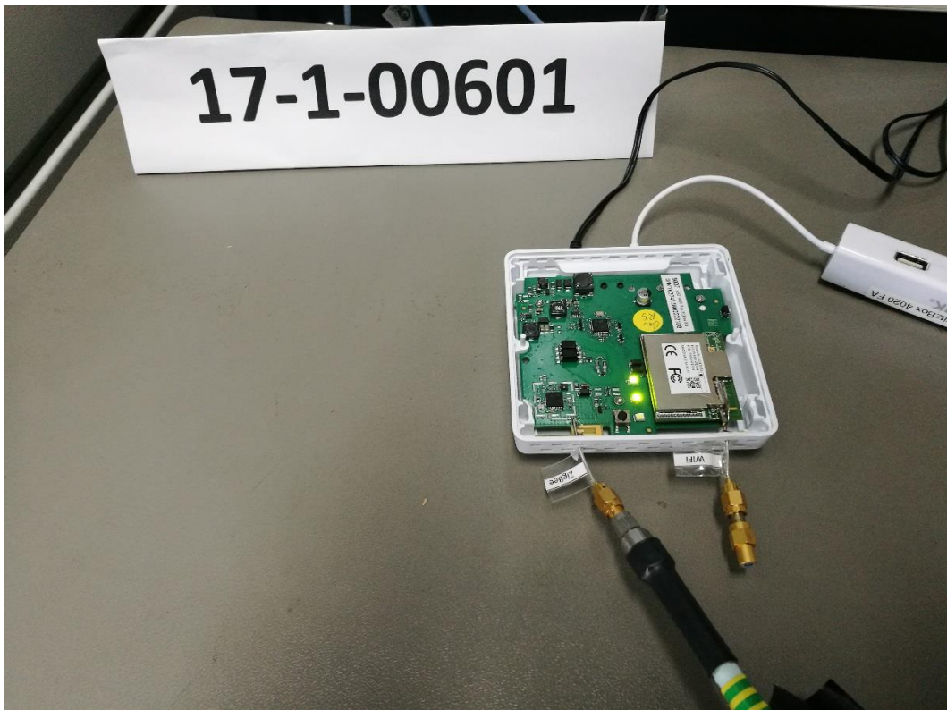
Photograph 4: Set Up 1-Close View -ZigBee 2.4 GHz Tests- RF Power + 20 dBc + 99% OBW
