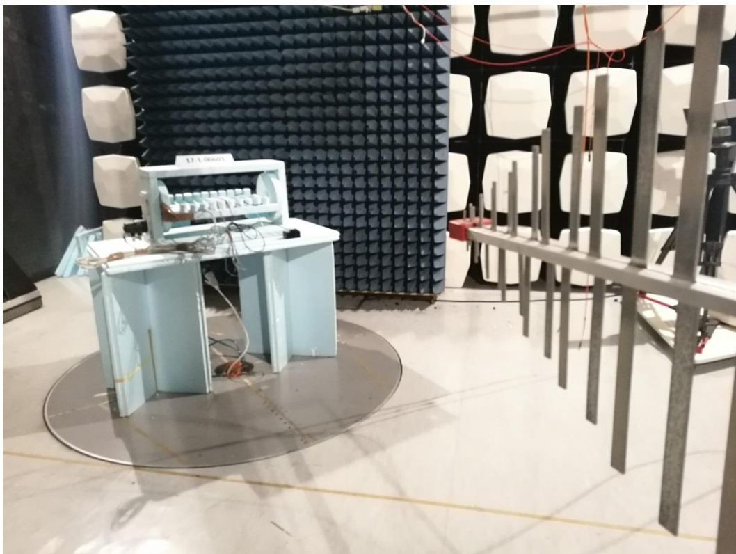
Photograph 8: Set Up 2-Overall View - 30 MHz-1 GHz - EUT Laying 0° - Front Side
