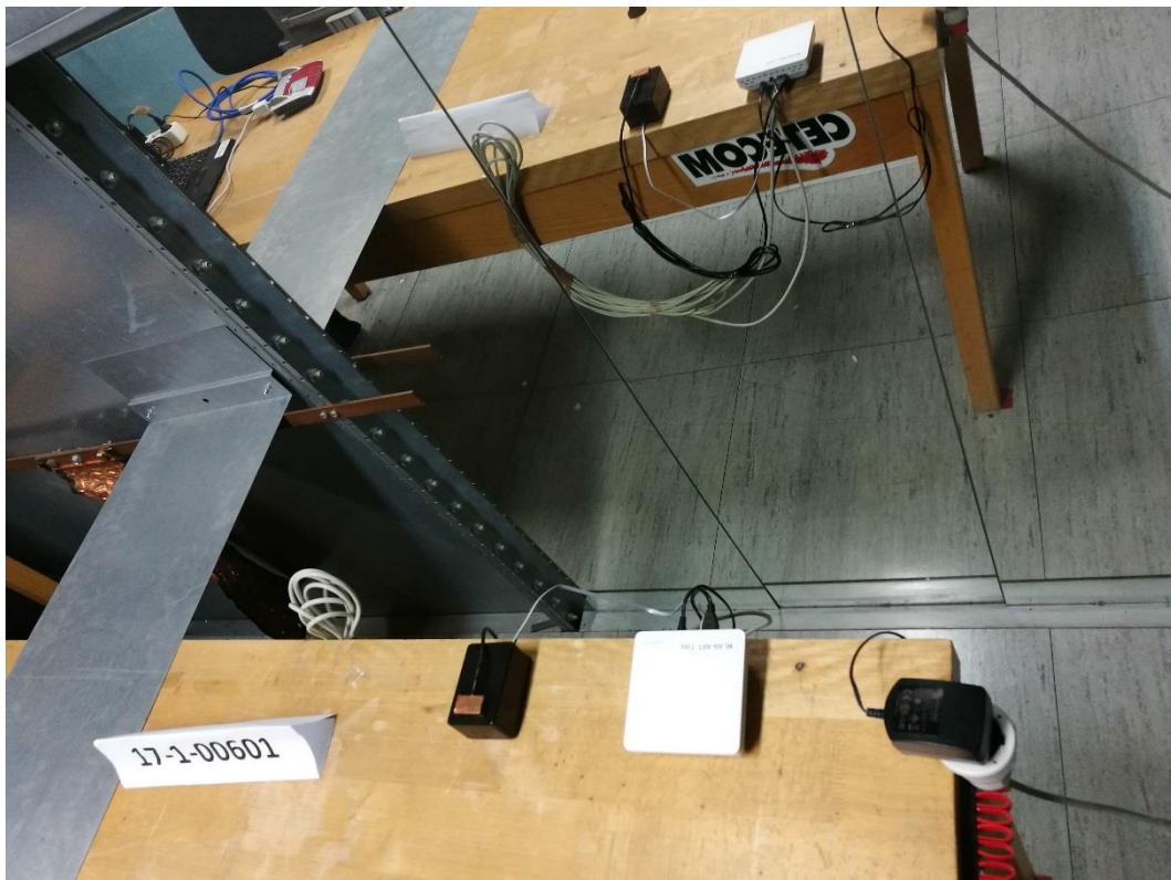
Photograph 15: Set Up 2-Close View -WLAN 2.4 GHz Tests- AC-Power Lines Emissions
