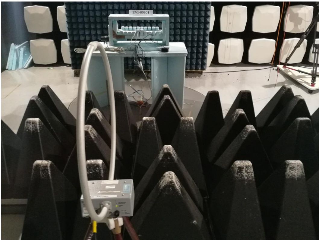
Photograph 4: Set Up 2-Overall View- 9 kHz-30 MHz- EUT Laying 0° - Front Side
