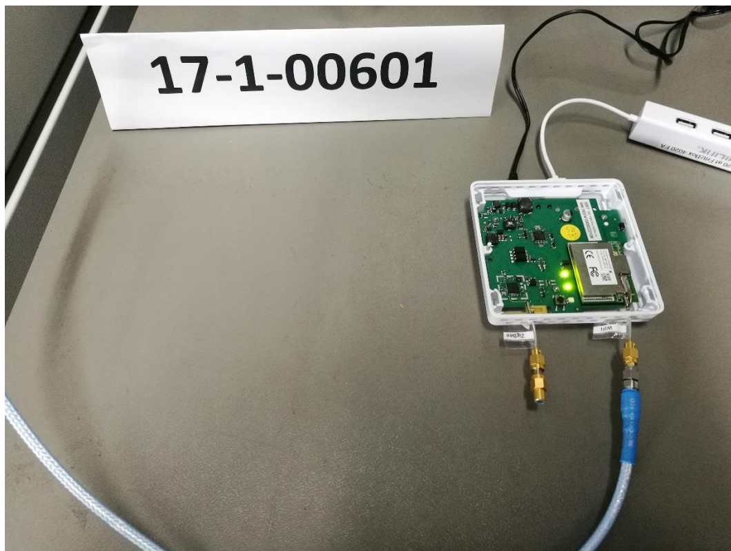
Photograph 2: Set Up 1-Close View -WLAN 2.4 GHz Tests- RF Power + Duty Cycle + PSD
