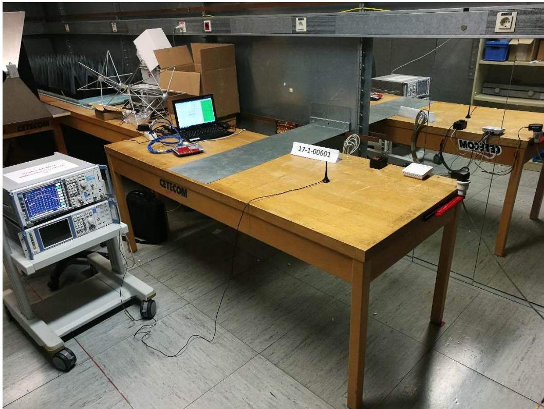
Photograph 14: Set Up 2-Overall View -WLAN 2.4 GHz Tests- AC-Power Lines Emissions
