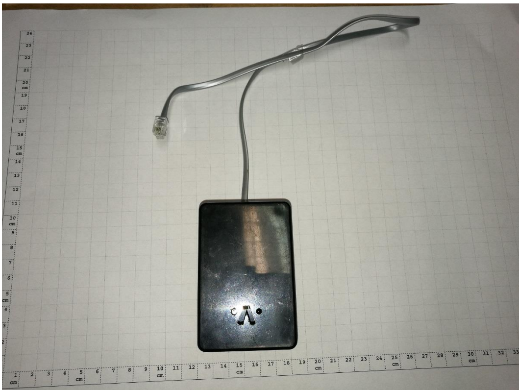
Photograph 8: AE 2 - Optolink Box with RJ10 UART Connection
