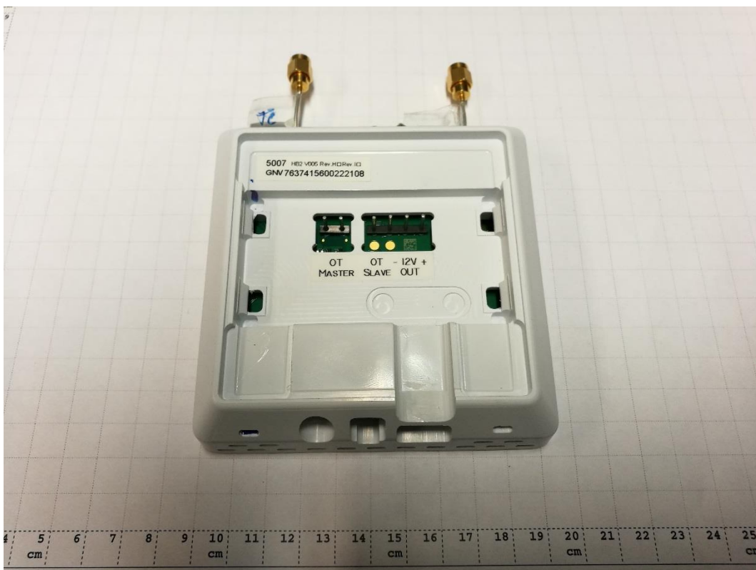
Photograph 6: Vitoconnect OT2 –Back Top Side with Conducted Connectors
