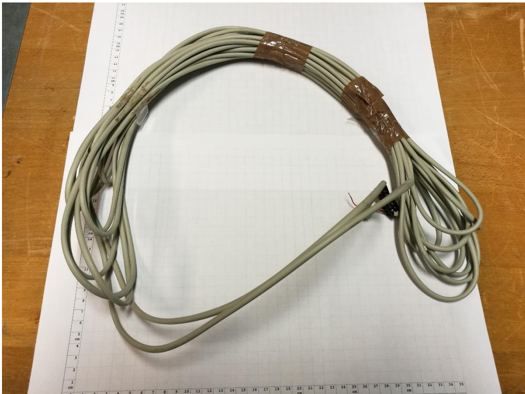
Photograph 10: AE 4 – Open Therm Loop Cable
