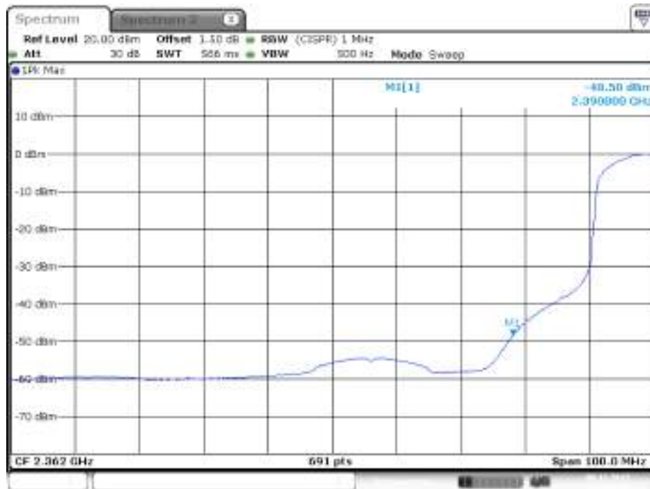
Plot on Configuration IEEE 802.11n MCS0 HT20 / 2412 MHz / Average / Chain 2
