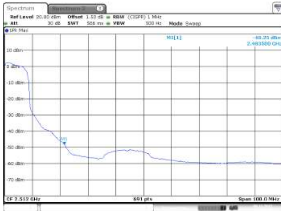
Plot on Configuration IEEE 802.11g / 2462 MHz / Average / Chain 1
