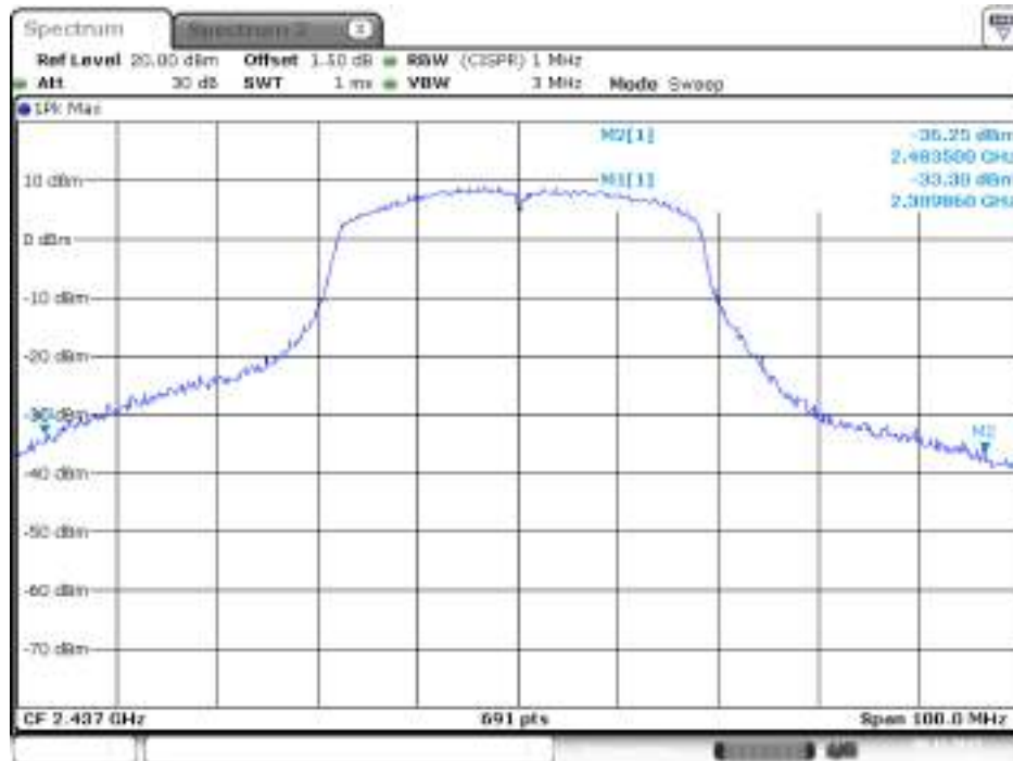
Plot on Configuration IEEE 802.11n MCS0 HT40 / 2437 MHz / Peak / Chain 2
