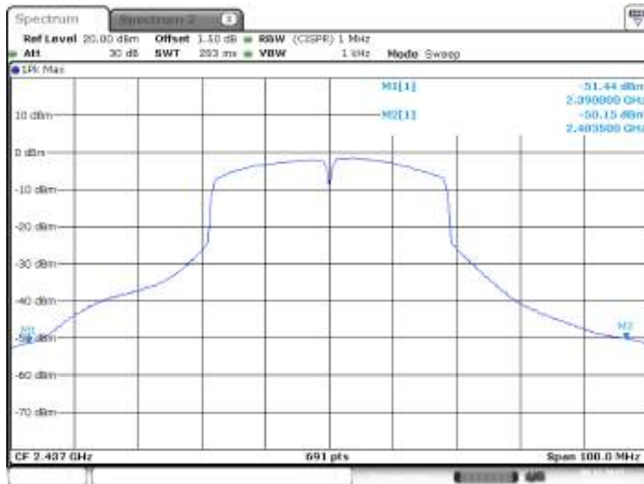
Plot on Configuration IEEE 802.11n MCS0 HT40 / 2437 MHz / Average / Chain 1
