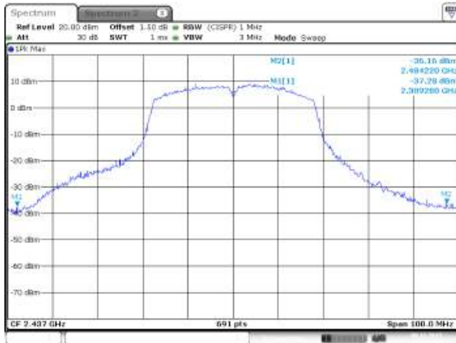
Plot on Configuration IEEE 802.11n MCS0 HT40 / 2437 MHz / Peak / Chain 1
