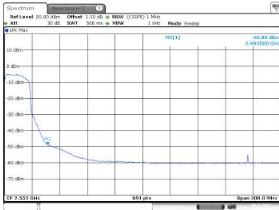
Plot on Configuration IEEE 802.11n MCS0 HT40 / 2452 MHz / Average / Chain 2
