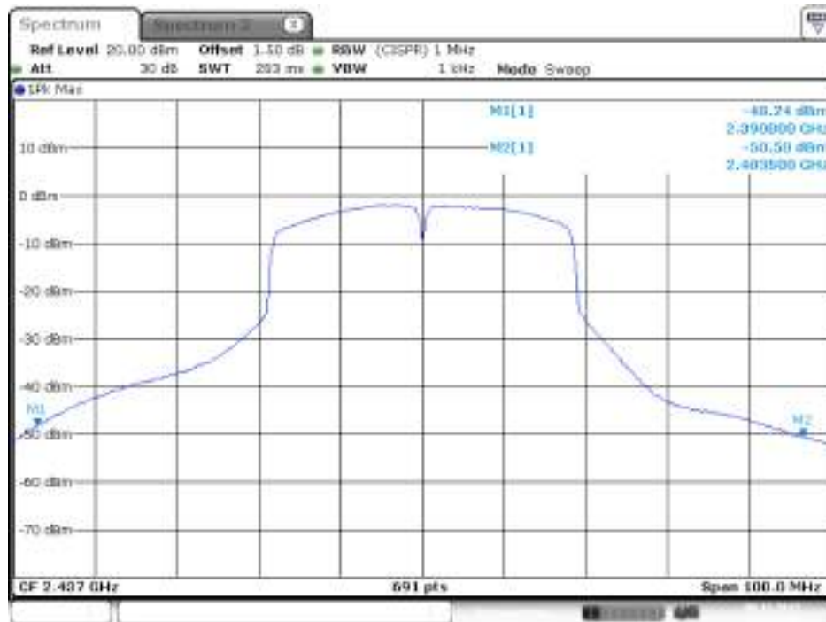
Plot on Configuration IEEE 802.11n MCS0 HT40 / 2437 MHz / Average / Chain 2
