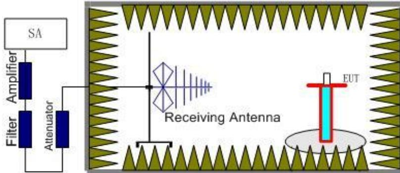
Radiated emissions measurements were made only at the upper, middle, and lower carrier frequencies. It was decided that measurements at these three carrier frequencies would be sufficient to demonstrate compliance with emissions limits because it was seen that all the significant spurs occur well outside the band and no radiation was seen from a carrier in one block of any band into
