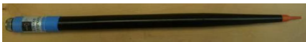
Figure 1 – MVG COMOSAR Dosimetric E field Dipole
