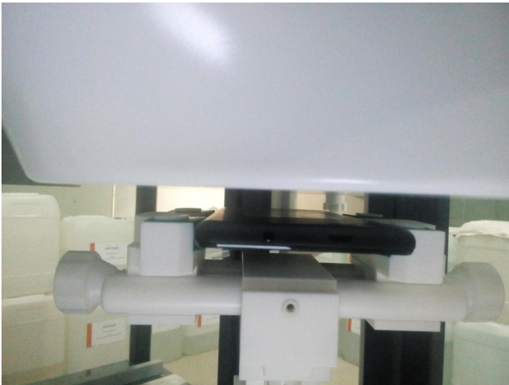
Body Back side(separation distance is 10mm)
