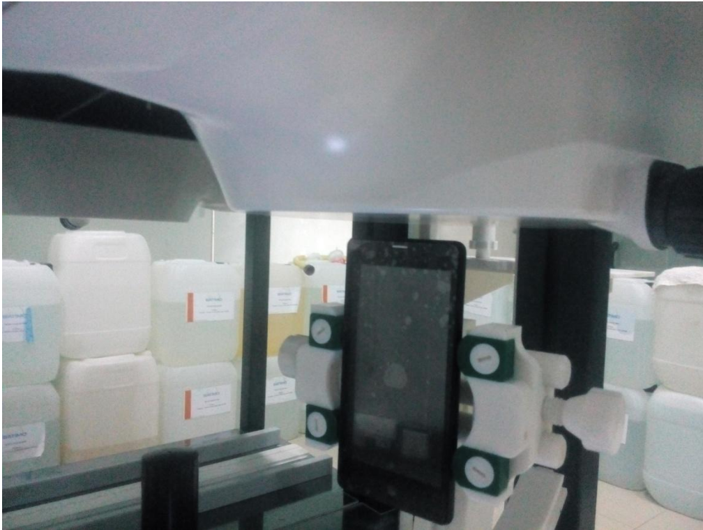
Body top side(separation distance is 10mm)
