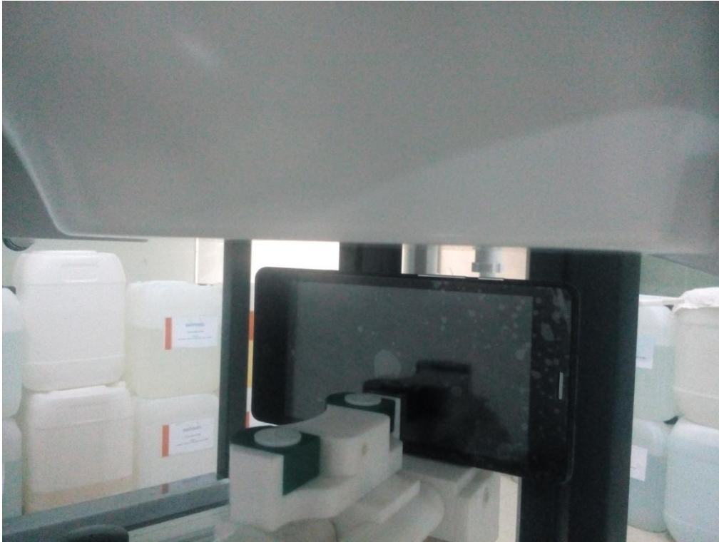
Body left side(separation distance is 10mm)
