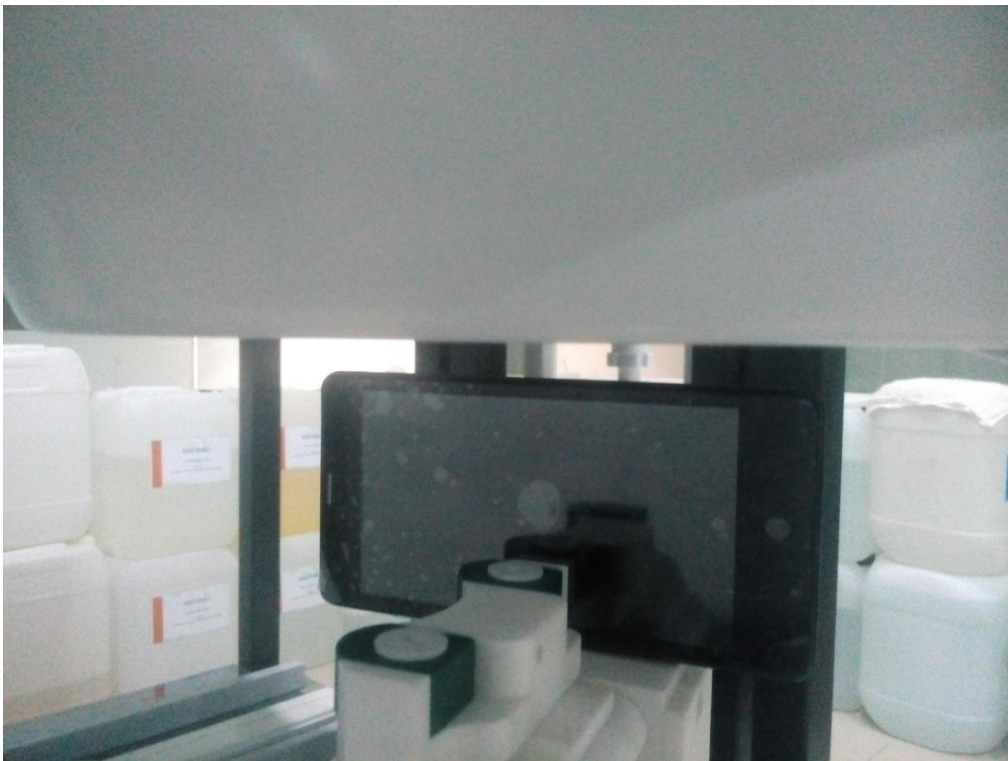
Body right side(separation distance is 10mm)
