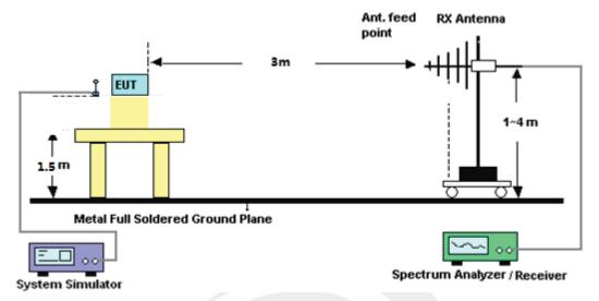
For radiated test from above 1GHz
