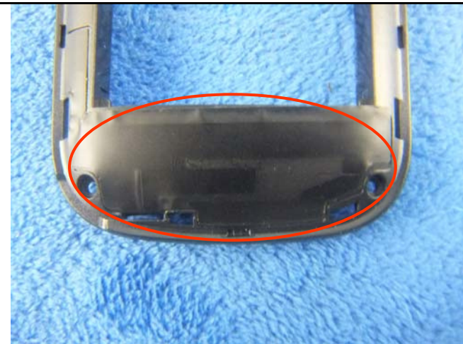
GSM/PCS Antenna View
