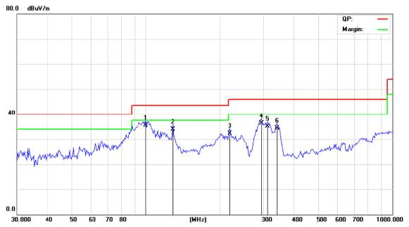
Site Chamber #2 Limit: FCC Part 15B Class B RE\_3 m Polarization: Vertical Temperature:
