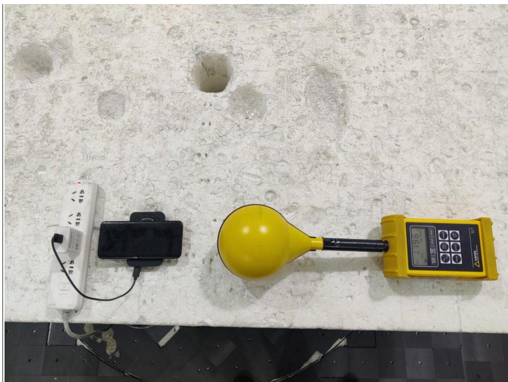
Test Position D - Exposure photo from side edge surface-Right(15cm) (TM1)
