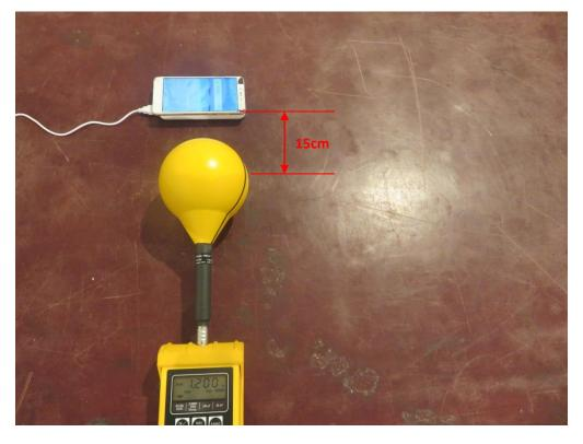
DUT – measurement position E – front side with 20 cm distance charging smartphone (SAMSUNG Galaxy S7)
