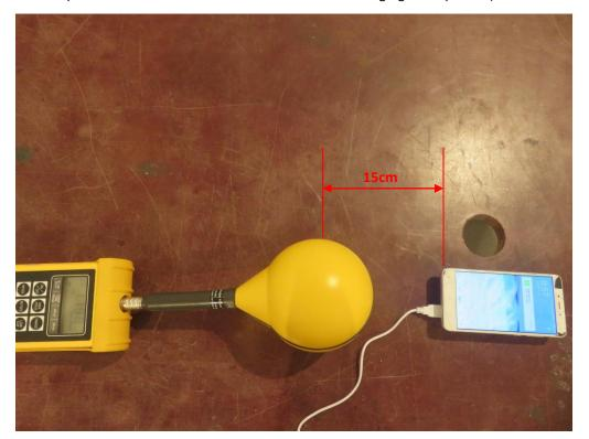
This report shall not be reproduced except in full, without the written approval of Shenzhen LCS Compliance Testing Laboratory Ltd. Page 6 of 9 DUT – measurement position D – right side with 15 cm distance charging smartphone (SAMSUNG Galaxy S7)
