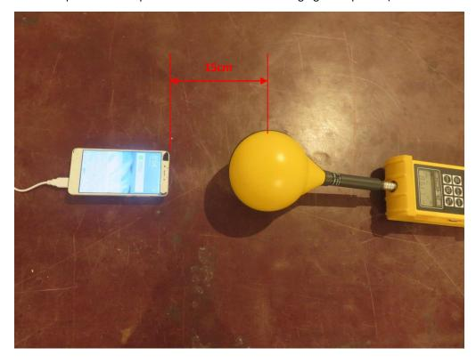
DUT – measurement position B – left side with 15 cm distance charging smartphone (SAMSUNG Galaxy S7)
