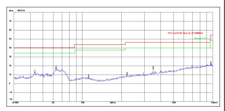
Site: Antenna::Vertical Temperature(C):24.8(C) Limit: **FCC Part15 RE-Class** Humidity(%):53.3%
