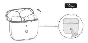
Open the cover of charging base when the headsets inside it, long press the button of charging base for 10 seconds, the indicator light flashes blue for 6 times quickly.
