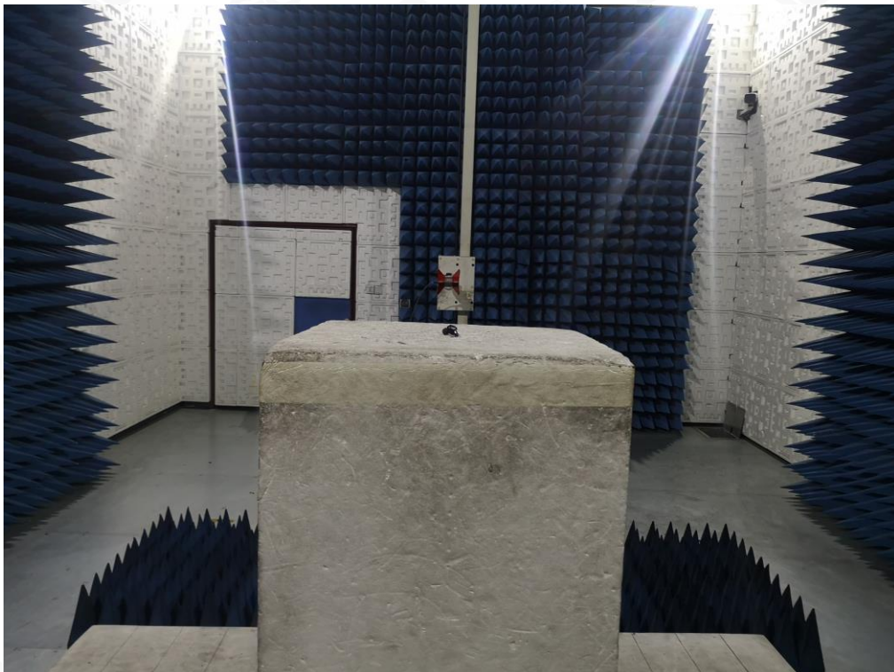
RADIATED EMISSION TEST SETUP ABOVE 1GHZ
